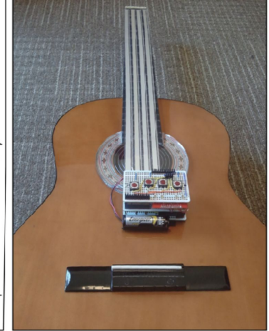
Figure 4: On the left is a Verplank Interaction Diagram, a framework for assessing different key aspects of a design. 13 On the right is the final project, a digital guitar with linear soft membrane potentiometers, to address the spatial sound control issues that the student had identified.
